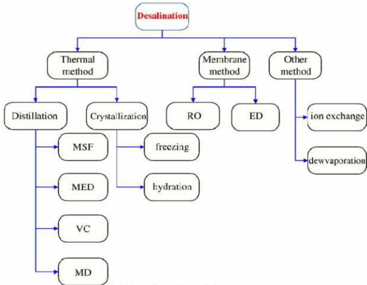
Fig. 1 Schematic diagram of the main desalination processes.
