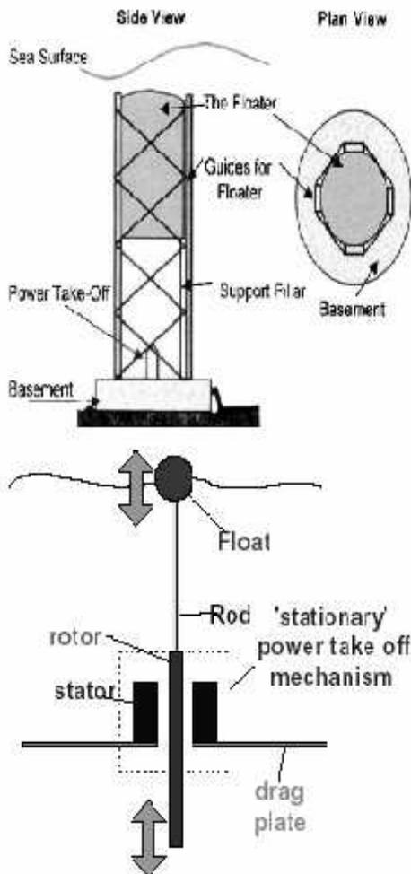
Fig.5 Archimedes Wave Swing
